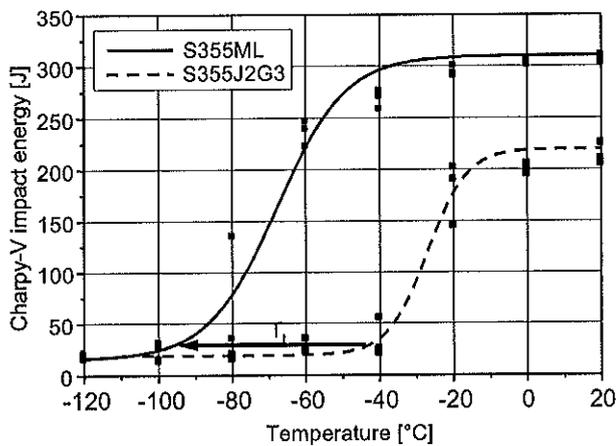
Figure 4. Comparison of the Charpy-V-temperature transition curve for a conventional normalized steel S355J2G3 and a TMCP rolled steel S355ML.
