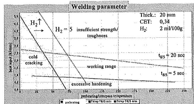
Figure 12.: Weld parameter box for S690Q, 20 mm thick.
