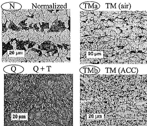
Figure 2. Microstructure of conventional normalised steel (process B of Figure 1) compared to TMCP (process D), TMCP+ACC (process F) and Q+T steel (process C).
