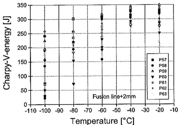
Figure 5. Charpy-V-temperature transition curve in the heat affected zone of a S355ML after welding with submerged arc welding ( $3.0 \text{ kJ/mm}$ ).
